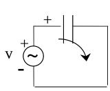
$$v_C = V_0 \cos(\omega t + \varphi_0) = \frac{q(t)}{C}$$
